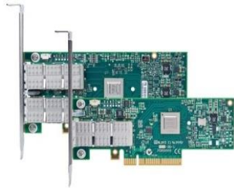
High Performance Interconnects – InfiniBand (with SR-IOV) <1usec latency, 200Gbps Bandwidth>
