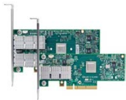
High Performance Interconnects – InfiniBand, Omni-Path <1usec latency, 100Gbps Bandwidth>
