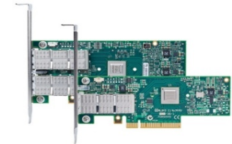
High Performance Interconnects – InfiniBand (with SR-IOV) <1usec latency, 200Gbps Bandwidth>
