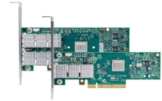
High Performance Interconnects – InfiniBand (with SR-IOV) <1usec latency, 200Gbps Bandwidth>
